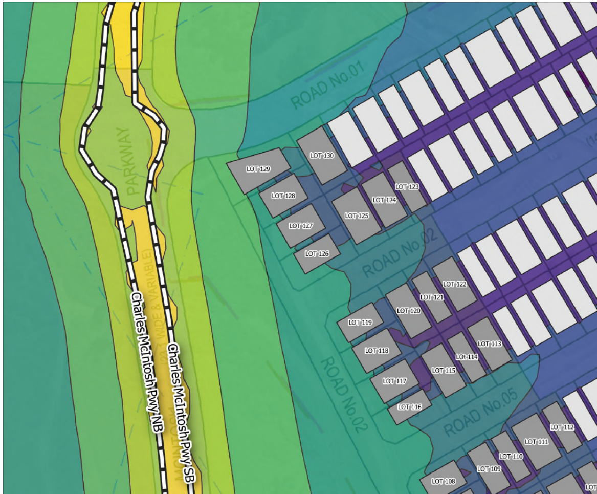
Figure 3: Extract of ground level noise contours (Lot 129)
